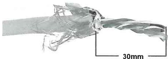
Strip approximately 30mm of the cable jacket, and separate to 4 pair each.
