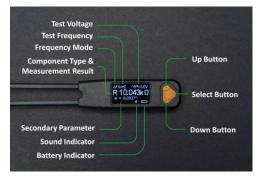
LCR Pro1 comes with a 0.96" OLED display, doubling the size of its predecessor's 0.91" display. The pixels are doubled as well from 128\*32 to 128\*64. Larger font and more information can be displayed for you to read the results and navigate the menu more conveniently.
