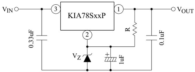
$V_{OUT} = V_Z + V_{OUT} \text{ (of IC)}$
