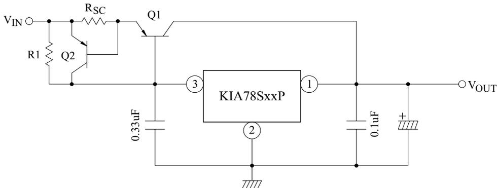
$$R_{SC} = \frac{V_{BE2}}{I_{SC}}$$
