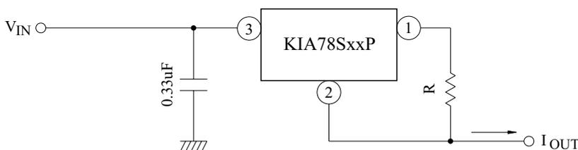
$$I_{OUT} = \frac{V_{OUT}}{R} + I_B$$
