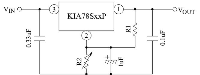
$$V_{OUT} = R_2 \left( I_B + \frac{V_{OUT} \text{ (of IC)}}{R_1} \right) + V_{OUT} \text{ (of IC)}$$
