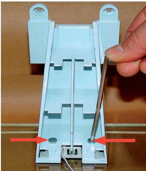
3. Use the hexagon wrench and two hexagon socket screws supplied to screw the base support onto the glass base. When doing this, make sure that the lighting cable from the device base is routed to the side as shown in the photo, so it does not become pinched.
