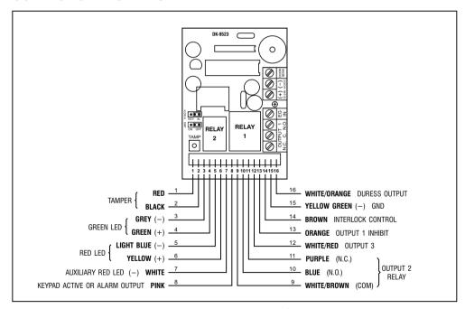
The connection facilities consist one set of terminal block mainly for Output 1 for door striking purpose; and one set of wire harness for Output 2 and 3, and the facilities for those auxiliary functions.
