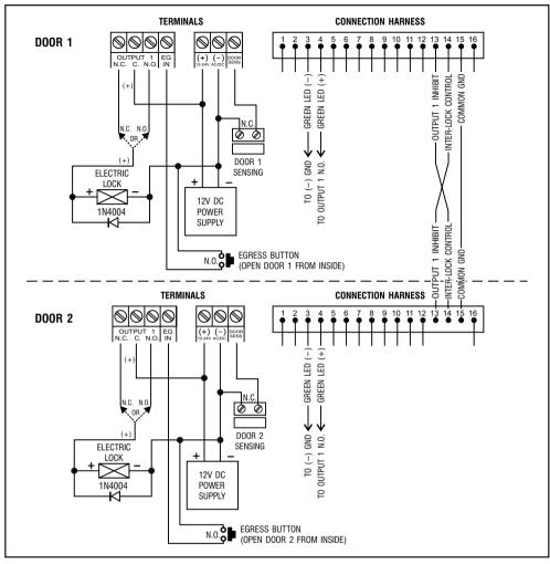
An inter-lock system needs two door controllers. This application example uses two DK-9523 with simple cross wire connection on their "Output 1 Inhibit" and "Inter-lock Control Output" terminals. It is necessary to link up the "(-) GND" terminals of the two keypads as common ground to achieve the inter-lock logical functions. The connection of the Green LED is optional. It will light up for lock active if connected.
