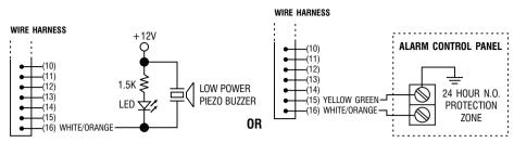
The Duress Output will switch to (-) ground when duress code is entered. You may use it to turn ON an LED lamp and /or a small buzzer to notify a guard; or connect it to a 24 hour Normally Open protection zone of an alarm system.
