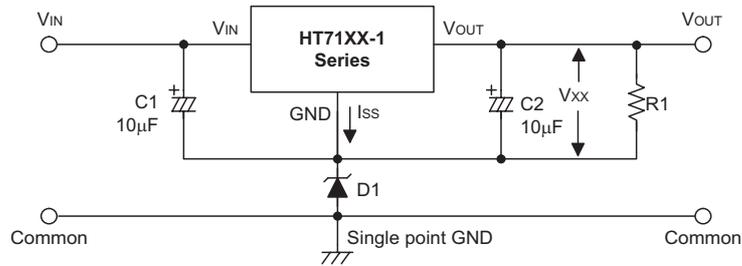
$$V_{OUT} = V_{xx} + V_{D1}$$
