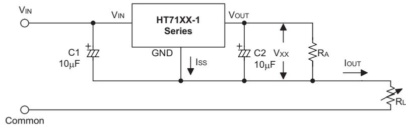
$$I_{OUT} = \frac{V_{XX}}{R_A} + I_{SS}$$
