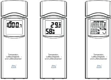
The indoor sensor displays room temperature and humidity, alternatively air pressure for the master sensor. The optional sensors (DNT000005) are addressable. The set address is displayed.
