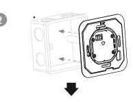
Screw the electronics in place using the enclosed mounting material.
