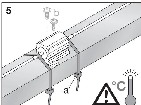
LEDDriving® CANBUS CONTROL UNIT must be fixed on a metallic surface. This can be achieved using the enclosed cable ties or separate special screws.\*
