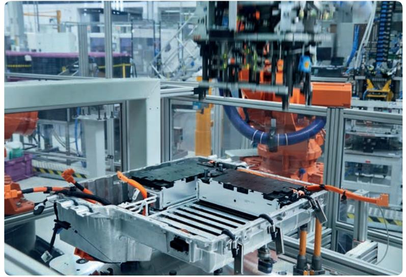
*The individual battery blocks are inserted into the sturdy metal housing by machine.*
