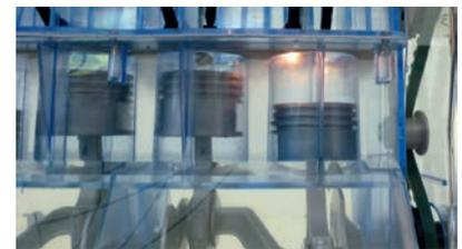
*Ignition too late: The fuel-air mixture is ignited when the piston is already on its way down.*
