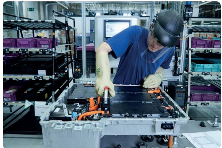
*In the next step, the individual battery blocks are wired together.*
