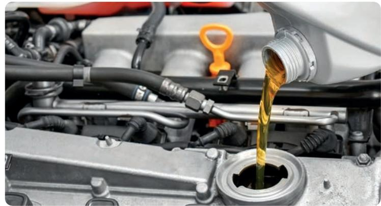
Engine oil reduces friction in the engine and also provides cooling for the moving parts. The oil film, for example between the piston wall and the inside of the cylinder, prevents the metals from rubbing against each other.
