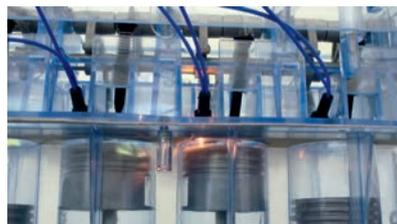
*With proper ignition timing, the ignition spark is visible when the piston reaches top dead centre. This way, maximum power is transferred to the piston.*
