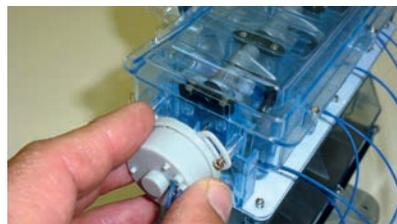
*Adjust the ignition timing of the model engine in several ways and notice where the piston is when ignition occurs. Also have a look at the valve positions.*
