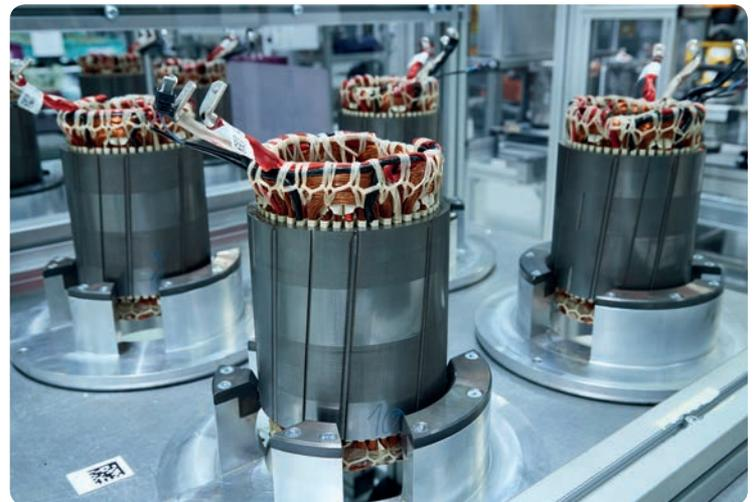
*Since the coil windings are also subjected to great mechanical forces, they are firmly connected to each other.*
