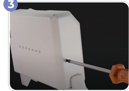
Step 6. Remove the hex screw in the lower left corner
