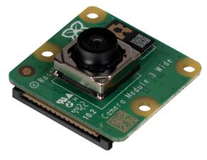
The Raspberry Pi Wide Angle Camera Module 3 is a compact camera for the Raspberry Pi, equipped with a 12 megapixel Sony IMX708 sensor.
