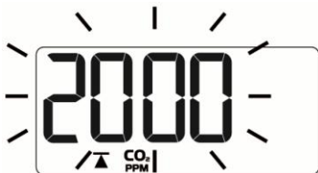
CO 2 high alert setting (default at 2000 PPM)
