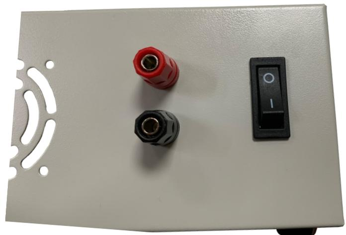
3. You can screw the black cable on the black bush and the red cable with the blade receptacle on the red bush. Therefore, you have to note that the cable lug is screwed before the washer and the other nut.
