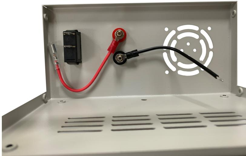
4. The cable must be now mounted with the blade receptacles on the switch. Therefore, you need to note that the cable from the bush is mounted on the position 0 and the other on position 1. Afterwards, insert the RD6006 into the case. You can affix the last loose cable ends on the module itself namely the current input terminal. Therefore, it is to note that the red cable must be screwed into the + and the black one into the -.
