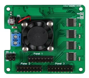
First plug the matrix controller board onto the GPIO bar of your Raspberry Pi. Connect the HUB75 connectors of your matrices with the corresponding connectors (panel 1, panel 2, panel 3) on the controller board.
