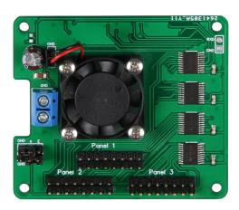
With the help of this expansion board for your Raspberry Pi you can control up to 3 RGB-LED-Matrix rows with the common HUB75 connector, e.g. our Joy-It RGB-LED-Matrix (LED-Matrix01). In addition, a 25x25mm fan is installed to ensure sufficient cooling of the Raspberry Pis.
