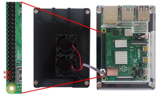
At this point, the case can be completely closed. All you have to do is place the cover of the case on the middle piece of the case. Then you are finished with the assembly of your RB-CaseP4+03B.
