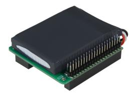
This battery hat turns the StromPi V3 into a full-featured UPS solution. The replacement battery is provided as third current source, is surveilled and will be recharged automatically.
