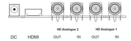
**DC:** Only use the 12v DC power supply included with the monitor.
