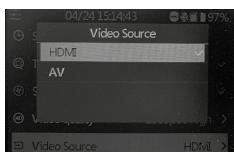
**Note:** AV input will automatically choose the recording resolution due to its original source (576p or 480p)
