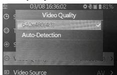
Video quality AV: 640x480. In the „Auto-Detection“ mode, the optimal resolution is automatically selected by the Grabstar PRO and the recording is saved in the format 720x576 or 720x480. It is not possible to influence the format during auto-detection mode.
