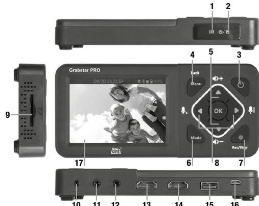
1 Remote control receiver (infrared)
