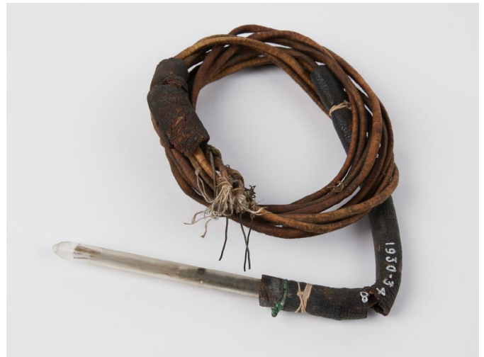
▲ Bild 1: Rectum-Platin-Thermometer by Callendar, 1886-1930 (Quelle)
