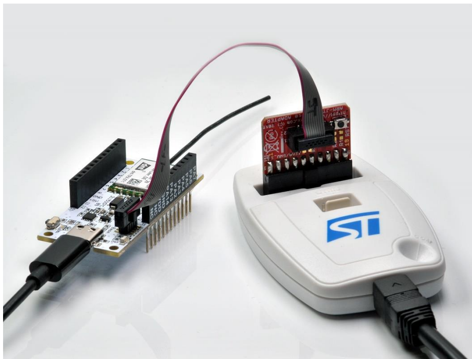
Figure 10: ELV-LW-Base completely connected
