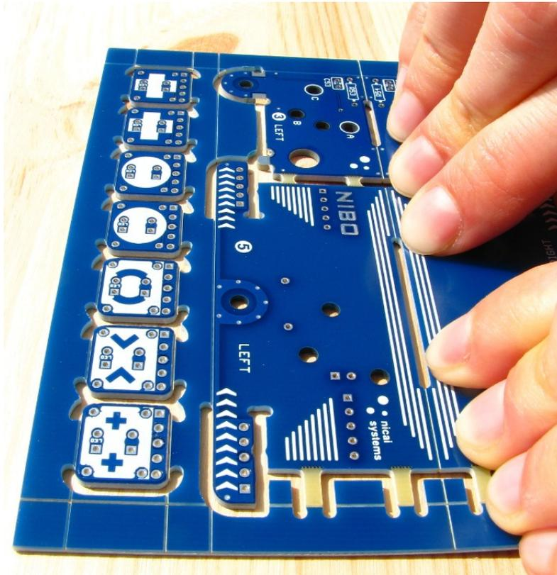
**Tip:** If you first **don't** separate the sensor brick boards, it is much easier to solder the electronic parts:
