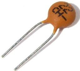
The both ceramic plate capacitors **C23** and **C24** have a capacity of 22 pF (imprint: 22).
