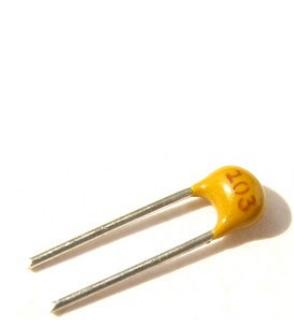
The **10 nF** ceramic multilayer capacitors (imprint: **103**) have to be placed into the soldering pads **C53** and **C54** on the **top sides** of the boards.
