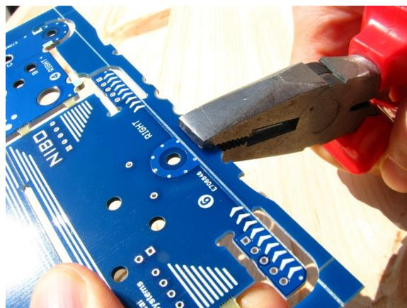
In order not to damage the single boards with the pliers, you can do the middle separation without it on a flat surface:
