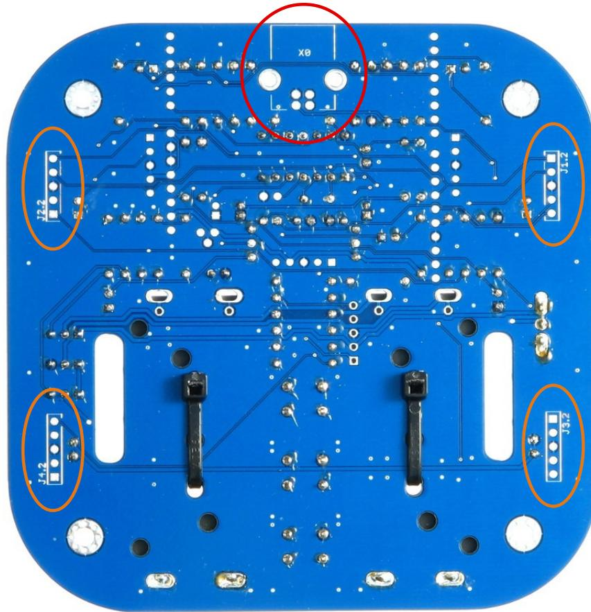
The straight 5-pin headers **J1.2, J2.2, J3.2, J4.2** and the USB socket **X0** have to be placed at this side of the board!
