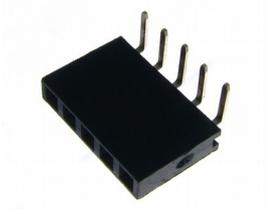
Four 5-pin right angle sockets have to be placed onto the **bottom sides** of the boards into the soldering pads **J1.B**, **J2.B**, **J3.B** und **J4.B**. They are soldered from the top side.
