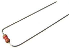
The little **mini!!** resistors with the value 2,2 k $\Omega$  (code: red-red-red- (gold)) have to be placed to the soldering pads **RB**:
