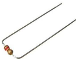
The little **mini!!!** resistors with the value 120  $\Omega$  (code: brown-red-brown- (gold)) have to be placed to the soldering pads **RA**:
