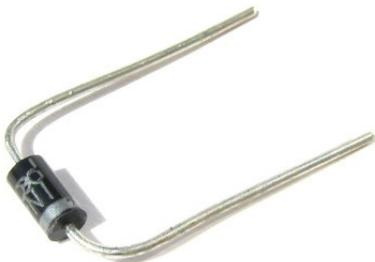
Also the Silizium diodes **D2-D9** of type **1N4007** must be bend like the resistors before placement.
