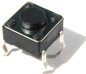
The placement of the buttons **SW1 - SW3** is protected against polarity reversal. You have to place it onto the board with soft pressure till it snaps in. You don't have to pay attention to the polarity.
