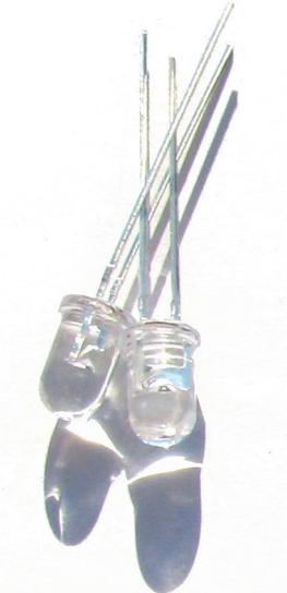
The leds **LED1** and **LED4** also have two legs: a short one (cathode) and a long one (anode).
