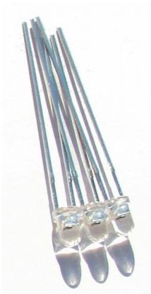
Place three **transparent** phototransistors into the **lower** soldering pads.
