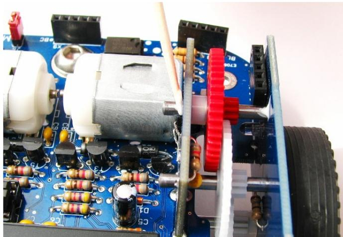
Additionally, the other axes can be greased.
