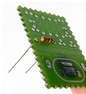
Now you have to heat the **soldering pad** and the **leg simultaneously** with the soldering iron at the bottom side of the board:
