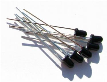
Place four black phototransistors into the **lower** soldering pads.
