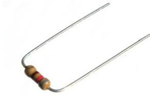
The resistors with the value **820  $\Omega$**  (code: grey-red-brown- (gold)) have to be placed into the soldering pads **R53** and **R54** on the **top sides** of the boards.
