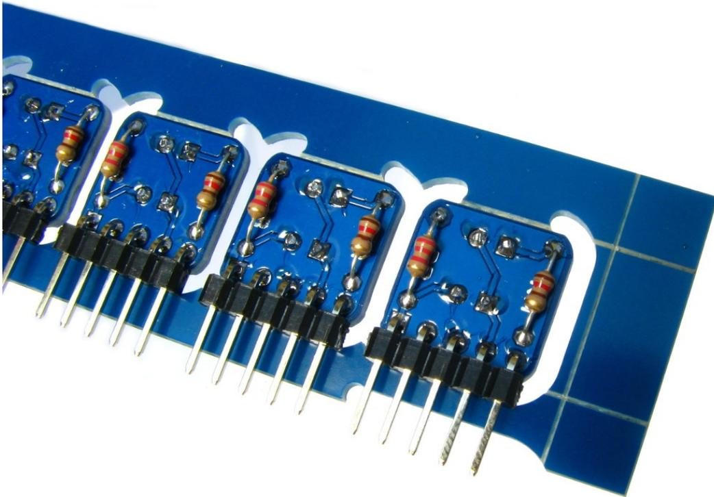
To get best sensor values it is advisable to shield **all phototransistors** with 3 mm long pieces of heat-shrinkable tubing:
