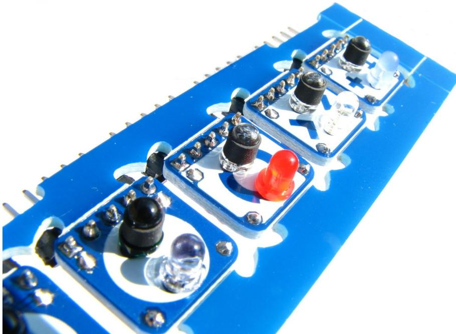
Now you can separate the individual sensor bricks from the frame:
