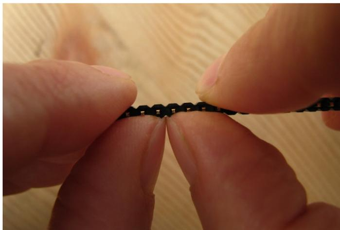
**Tip:** To count correctly it can be helpful to place a 5-pole socket onto the header before breaking.
