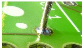
The leg of the electronic part has to be fixed at the soldering pad. If it is not yet fixed, you have to solder again!
