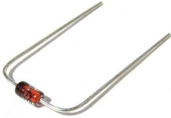
The Zener diodes **D20** and **D21** of type BZX83V003.6 (respectively 55C3V6) and the Schottky diodes **D1**, **D22**, **D23** and **D24** of type BAT85 must be bend like the resistors before placement.
