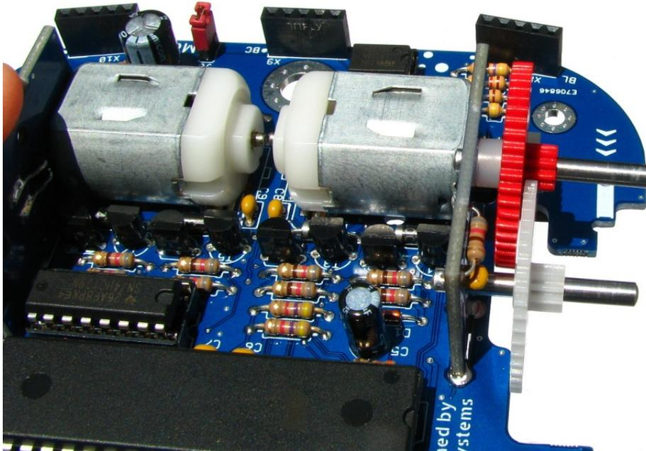
Then the **long axis** with the **white** gearwheel (the little gearwheel outwards) must be put into the **lowermost borehole**:
