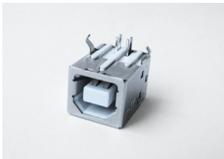
During installation of the USB socket **X0** you should pay attention that the smaller pins are not bent. The part is polarity safe. The USB socket is soldered at large at **6 soldering pads**.
