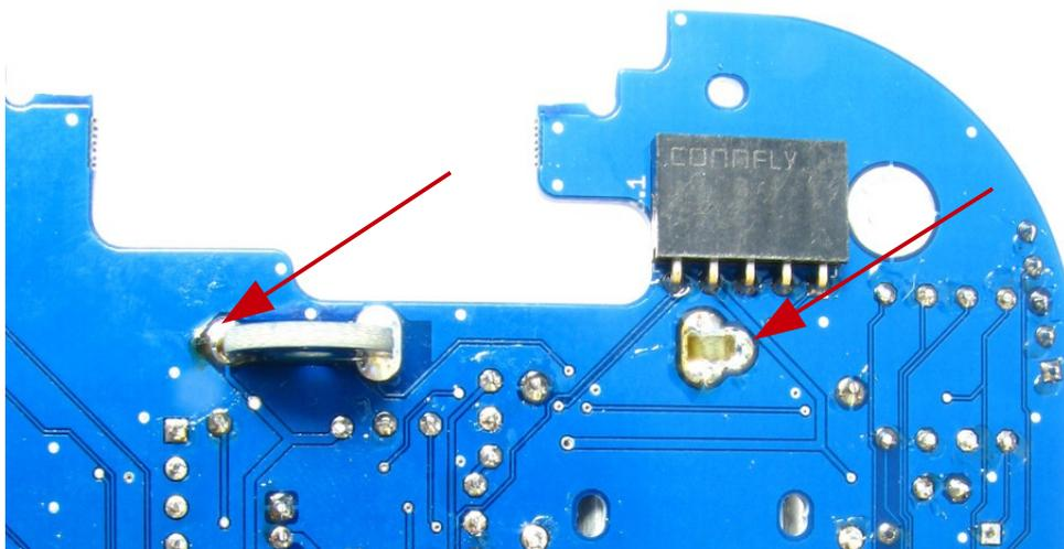
Then the motor contacts have to be soldered to the board:
