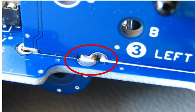
Now the both remaining connections (red arrows) must be soldered from the **bottom side** of the main circuit board.
