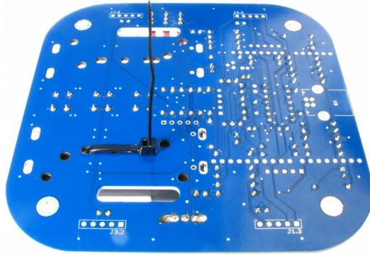
The cable strap has to be **cut shortly** with an electronic cutting pliers.
