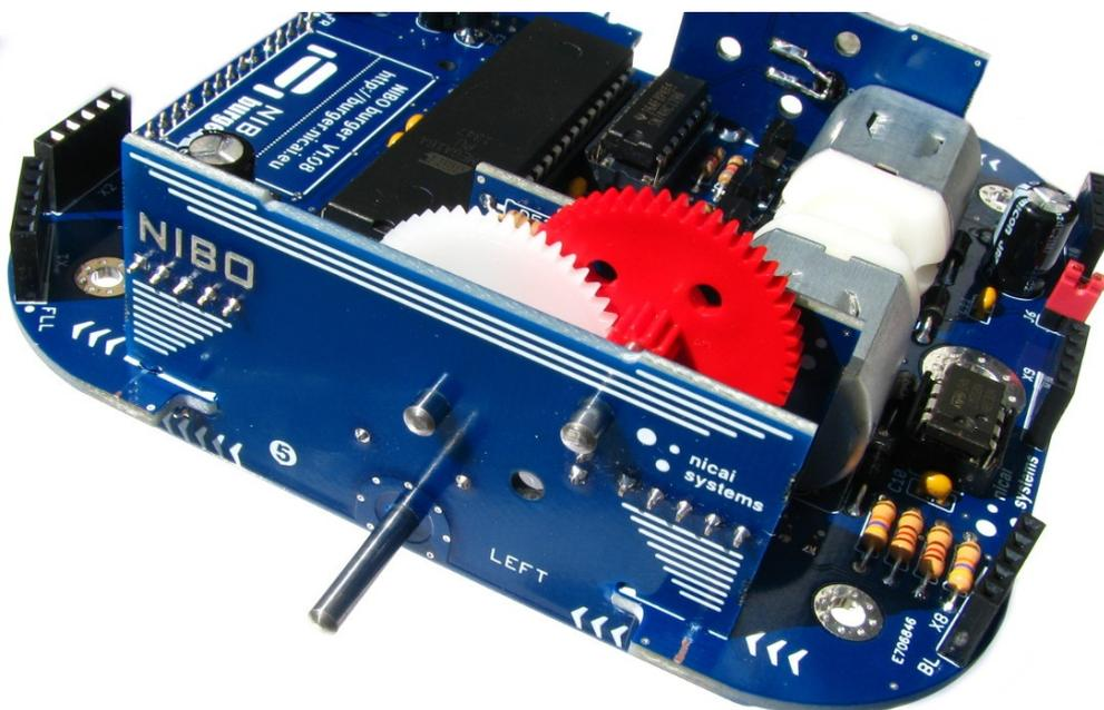
The 5-pin headers must be connected to the 5-pin sockets of board ①:
