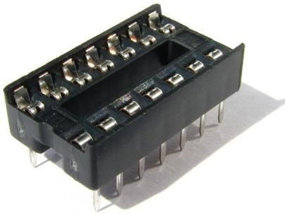
There are **four** IC-sockets to be soldered onto the boards. The 40 pin socket is for the main controller ATmega16, the **14 pin** socket is for the ATtiny44, the **16 pin** socket is for the demultiplexer 74HC139 and the 8 pin one is for the operational amplifier LM358.
