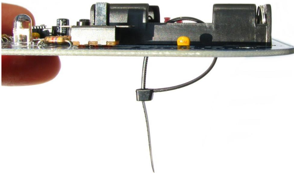
Then the cable strap is to be fastened (e.g. with an universal pliers):
