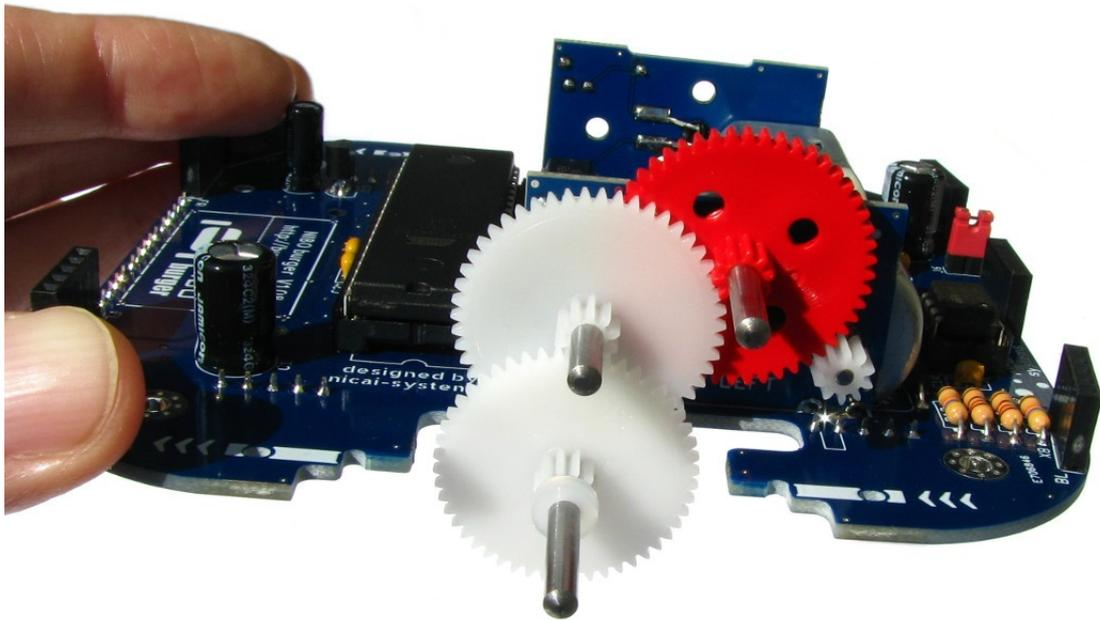
The transmission is fixed by board ⑤ (the electronic parts of board ⑤ point inwards):
