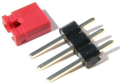
The 3-pole jumpers **J1**, **J2**, and **J3** have to be soldered analog to the 2-pole ones. After soldering the jumpers must be connected at the **RUN** position.
