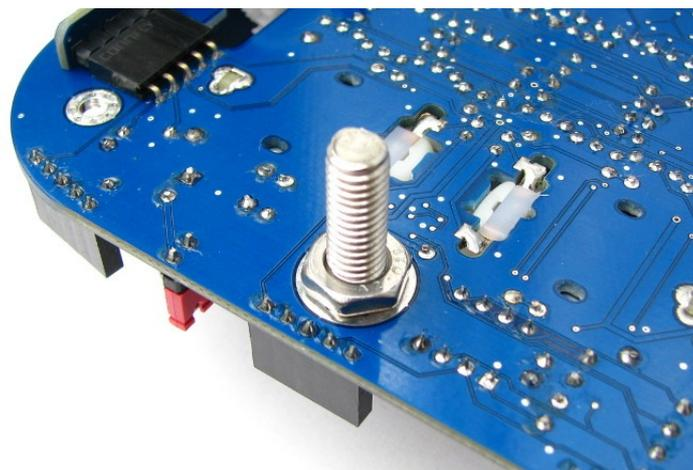
Finally the white polyamid pin must be screwed on:
