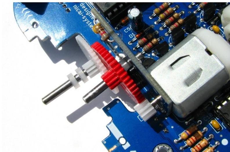
**Note:** For this transmission unit setting it is necessary to bend the both transistors nearby the short axes a little bit:
