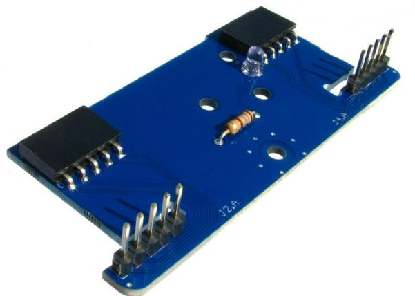
Later on the side plates have to be plugged with other plates. Therefore it is important to solder the headers at **right angle** onto the boards:
