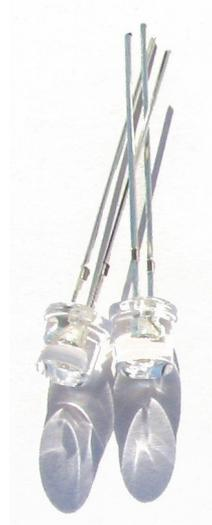
The leds **LED2** and **LED3** also have two legs: a short one (cathode) and a long one (anode). The body of these components is flattened.
