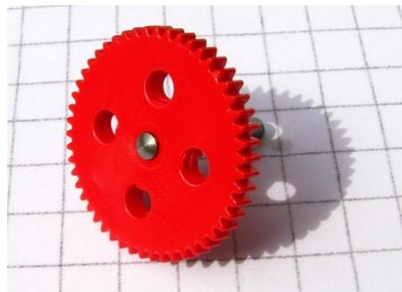
Then you have to press the axis **carefully** through the gearwheel. For not getting injured, the **thumbnails** must have some **distance** to the axis:
