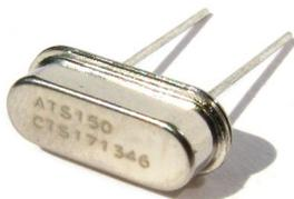
The crystal **Q1** has a frequency of 15,000MHz and must be placed on board ②. After positioning the body should not be in contact with the board (Optimal distance to the board: 1mm).
