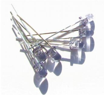
Each board gets one IR led. They have to be placed into the marked soldering pads (see the photos).
