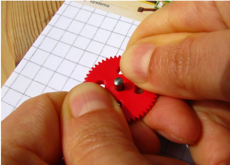
Afterwards the gearwheels should be in the middle of the axis:
