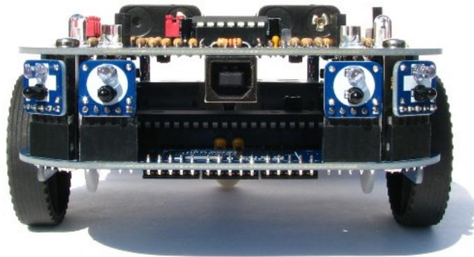
The **colour sensor bricks** must be put into the bottom slots in the **following order** (BR - red, BC - green, BL - blue):
