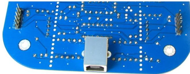
...and solder it at the **top side** of the board at **6 soldering pads**, the two holders of the housing have to be completely filled with tin solder:
