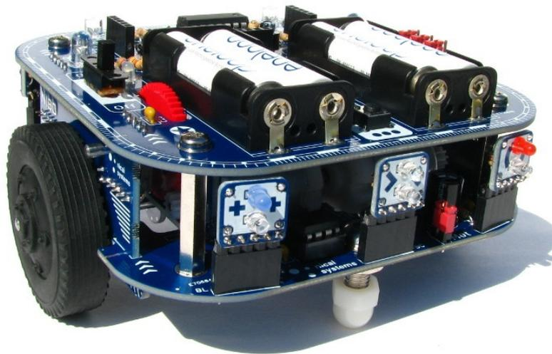
You can also plug the 3 sensors into the slots at the bottom side of the robot to analyse coloured floors. This setup is also well suited for following lines.
