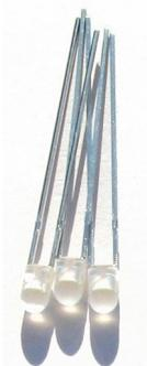
The LEDs **LED5 - LED7** have got two legs, a short one (cathode) and a long one (anode).
