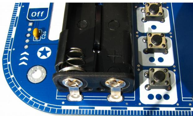
**Before** soldering the battery packs must be fixed with the small cable straps at the circuit board.
