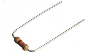
The resistors are soldered horizontal onto the boards. The legs must be bent over, as shown in the illustration.
