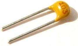
There are 13 ceramic multilayer capacitors to be placed onto the board.
