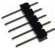
Finally four 5-pin straight headers are placed into the soldering pads **J1.A**, **J2.A**, **J3.A** and **J4.A** from the **bottom** sides of the boards and are soldered from the top sides.
