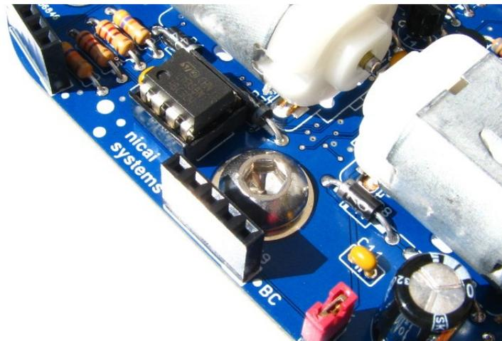
Then the screw is fixed from the bottom side with a hex nut:
