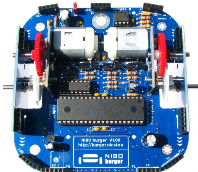
**Tip:** You can reduce the operating noise by careful greasing the transmission (see also page 82).
