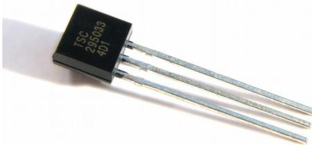
The 3,3 V voltage controller IC must be placed onto board ① into the soldering pad **IC3**.
