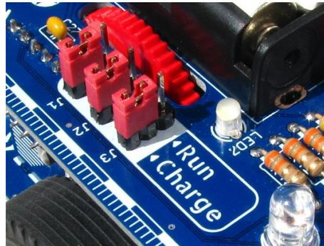
The **white LED 7** (shown on the photos) indicates the **state of charge**:
