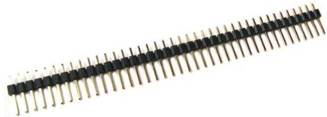
Because all headers must be **separated** to **5-pin** configuration, you have to count 5 contacts and break the strip with the thumbnails at the right position:
