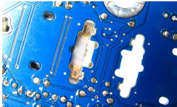
For an easier soldering of the motor contacts and board ① you can bent up the motor contacts a little bit.
