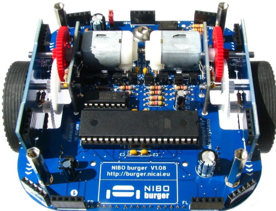
Now we connect board ② with the side boards in the **right orientation!!** and fix it with four screws.
