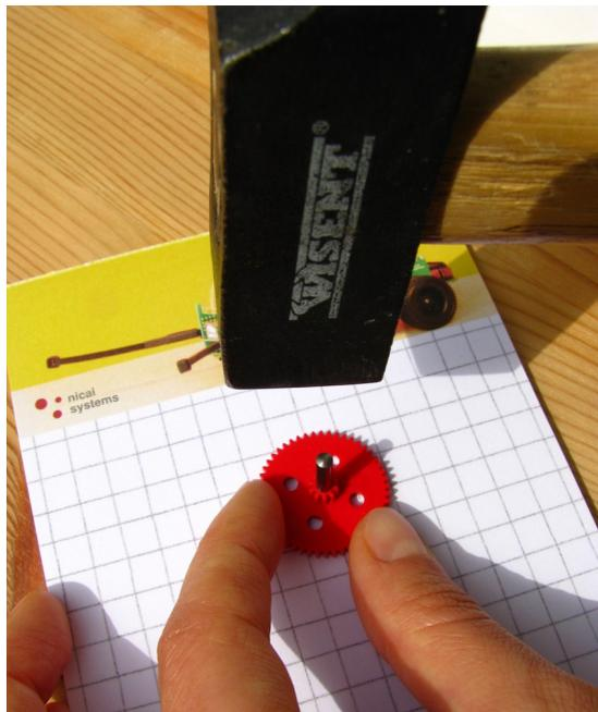
The axis must be pressed through with the hammer until it looks like this:
