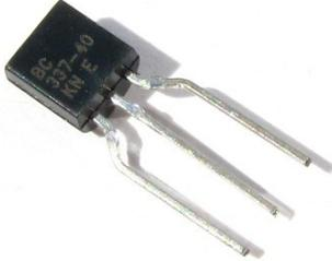
The five NPN bipolar-transistors **T3, T4, T5, T6** and **T9** are of the type **BC337 !!**.
