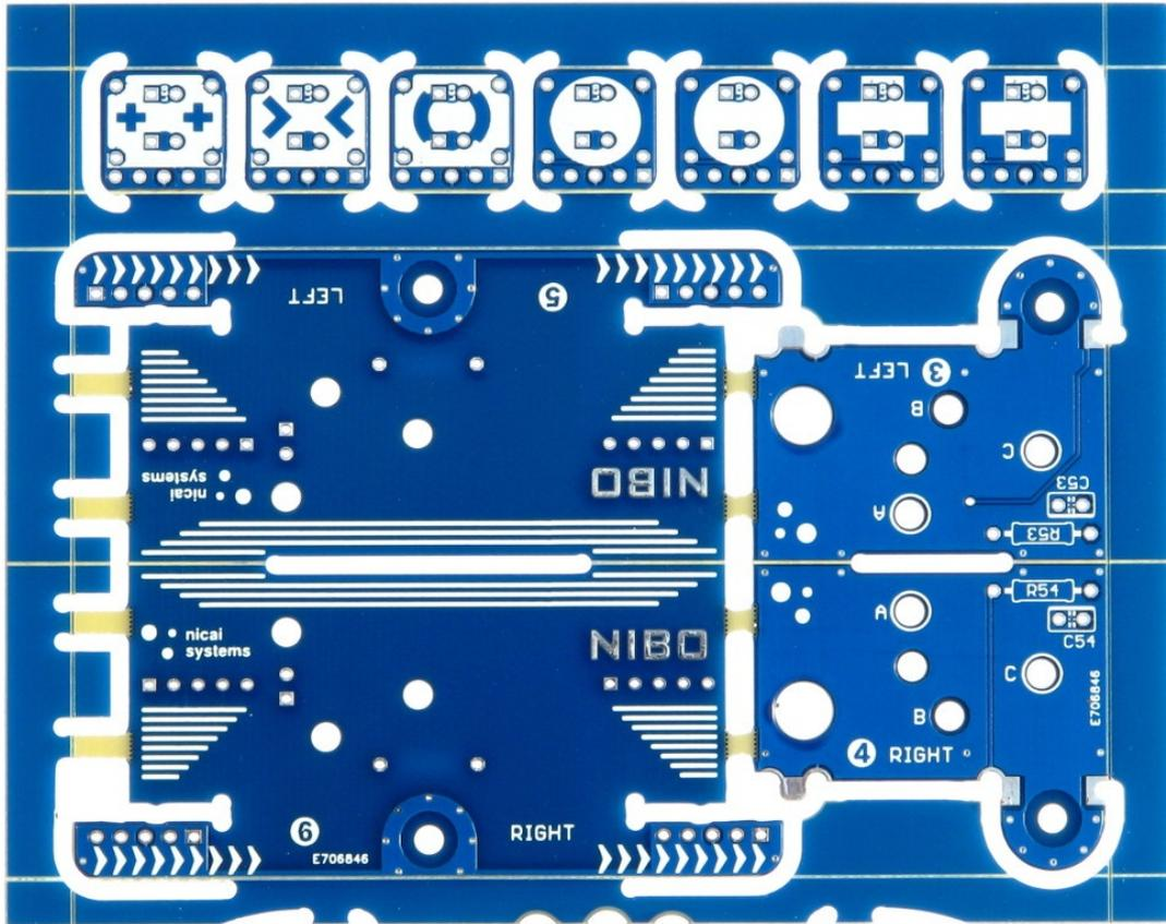
At first the boards ③ - ⑥ (**NOT the sensor bricks!**) must be separated from the frame e.g. by an universal pliers:
