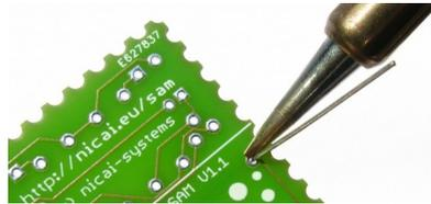
Then the **tin-solder** has to be attached **additionally**. If everything is well heated, the tin-solder is melting and the leg of the electronic part gets connected to the soldering pad:
