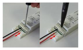
To wire the FLS-PP lp use conductor with crosssection of  $0.2-0.75 \text{ mm}^2$  (AWG24–18). Dismantle the cable 6–7 mm.
