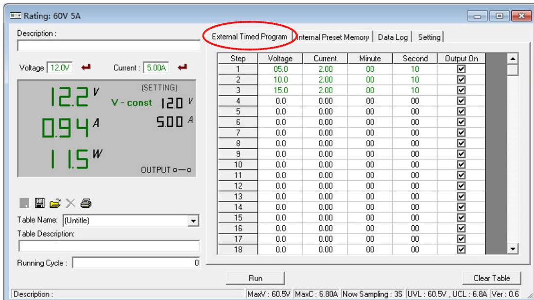
External Timed Program is completely controlled by PC, PC counts the time and changes voltage and current of power supply.
