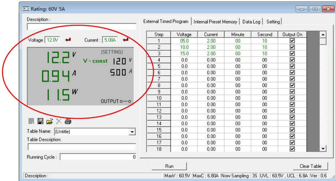
1. You can directly type the desired output voltage & output current and then click enter symbol to set the value
