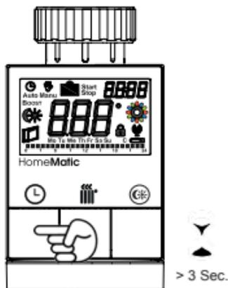
Menu items can be selected with the handwheel and confirmed with the Boost button (⚙️). By pressing the Auto/Menu button (⌚) again, you can return to the previous level. The display will change back to normal if changes have been made successfully. The menu automatically closes without applying changes if there is no operation for more than 1 minute. The following settings can be made:
