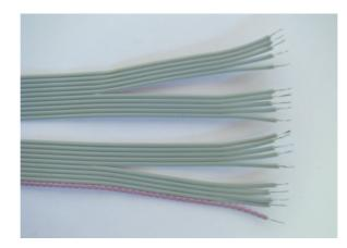
The conductors must be soldered in the numeric order to their corresponding pads on the display-board:
