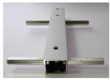
The next step is to mount the OMS-boards to both sides. Therefore you have to place the square-profile as shown in the image (page 16). The top side of the square-profile can be easily identified: the large boreholes for the motors are closer to the top side of the profile.
