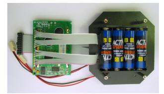
If required the batteries of the bottom side can be fixed by the enclosed cable ties. Therefore the two cable ties have to be spanned through the four remaining boreholes around both battery packs.
