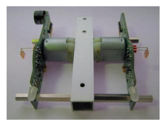
The red and the black cable must be cut into halves. The four pieces must be isolated 0,5 cm on one side. Afterwards they can be soldered from the outside to the OMS-boards:
