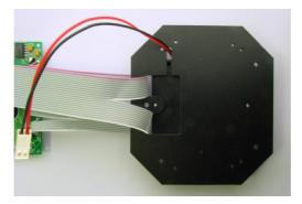
The second battery pack has to be screwed from the **bottom side** of the plate at the boreholes (**3**).
