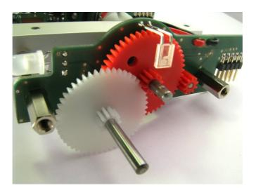
Now the transmission is fixed with one aluminum cover panel and two hexagon socket screws. The same procedure applies to the other side.
