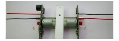
Now the cables must be put inwards through the holes and soldered to the motors (see the photo). Therefore you have to shorten and isolate them.
