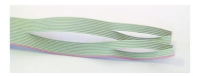
Now each conductor needs to be separated (approx. 2 cm), isolated (approx. 5 mm) and tinned. Afterwards you may solder five conductors in each step.
