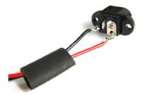
Afterwards you have to isolate the connections with the heat-shrinkable tubing:
