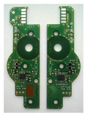
The finished component side (top side) of the boards should look like this:
