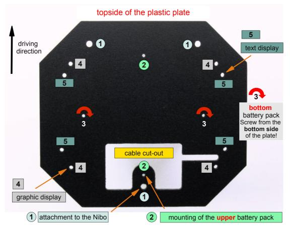
Now the complete 2<sup>nd</sup> floor has to be screwed onto the distance bolts of the engine section at the boreholes (1) with three hexagon socket screws. Before it is advisable to **switch-off the robot** (toggle switch backward), to put all connectors into the corresponding sockets and to place the cables optimal.
