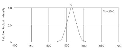
$\label{eq:wavelength} \mbox{wavelength} \ \ \, \mbox{$\wedge$ (nm)$} \\ \mbox{RELATIVE INTENSITY Vs. WAVELENGTH}$
